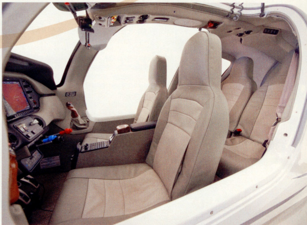
The airplane's interior is well-appointed, but without fuss. Back-seat passengers have a satellite music jack, and the front seats seem roomy, thanks to the lack of a yoke (above). The Garmin G1000 keypad sits below the center armrest, making inputs quite easy. Overhead switches (top) give a large-airplane feel, and further reduce panel clutter.
